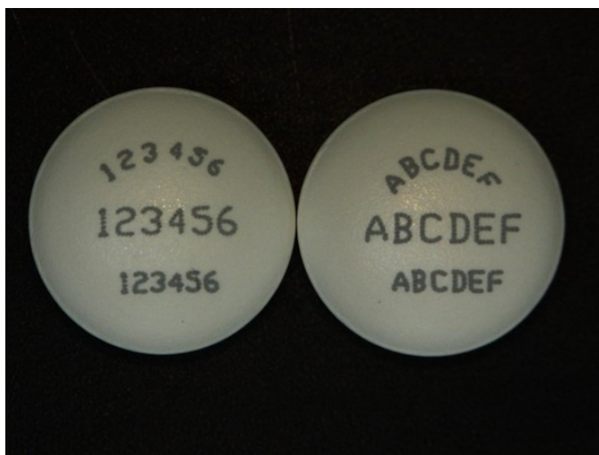
Photograph of Tablets Printed with the UV Laser Irradiation Technique.
