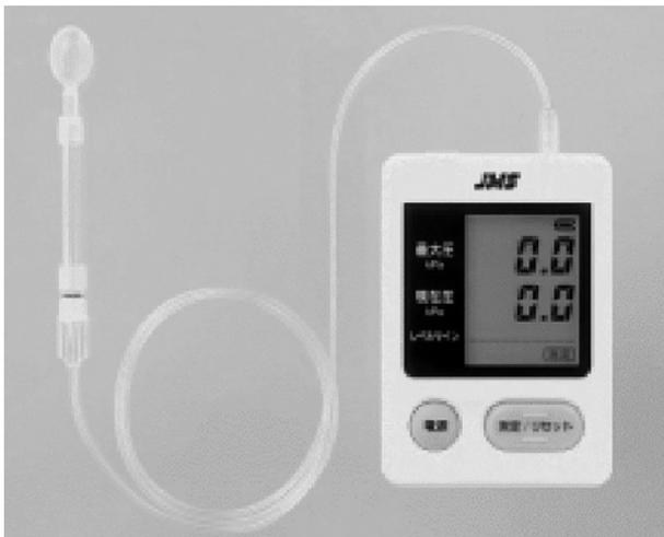
Fig. 2 Tongue pressure measuring device (TPM-01, JMS, Hiroshima)
