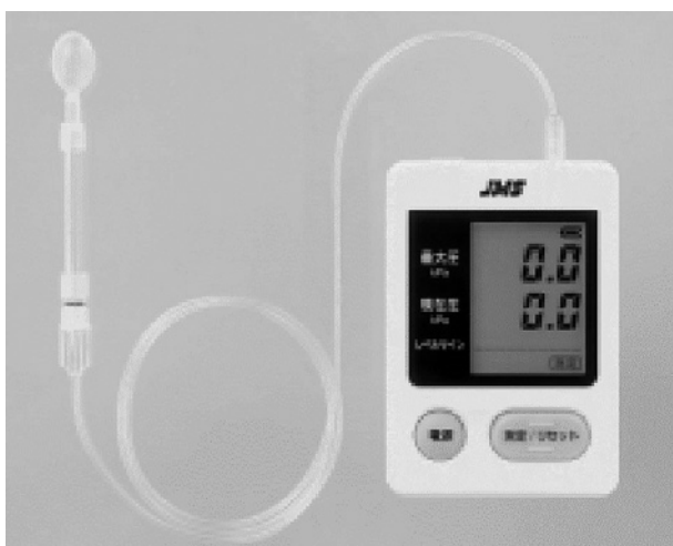
Fig. 2 Tongue pressure measuring device (TPM-01, JMS, Hiroshima)
