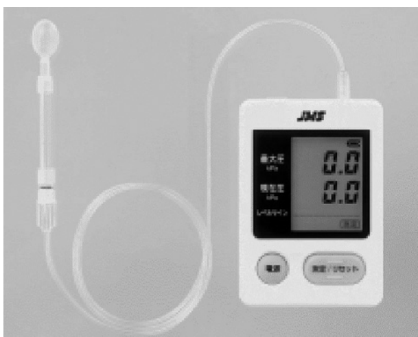
Fig. 2 Tongue pressure measuring device (TPM-01, JMS, Hiroshima)
